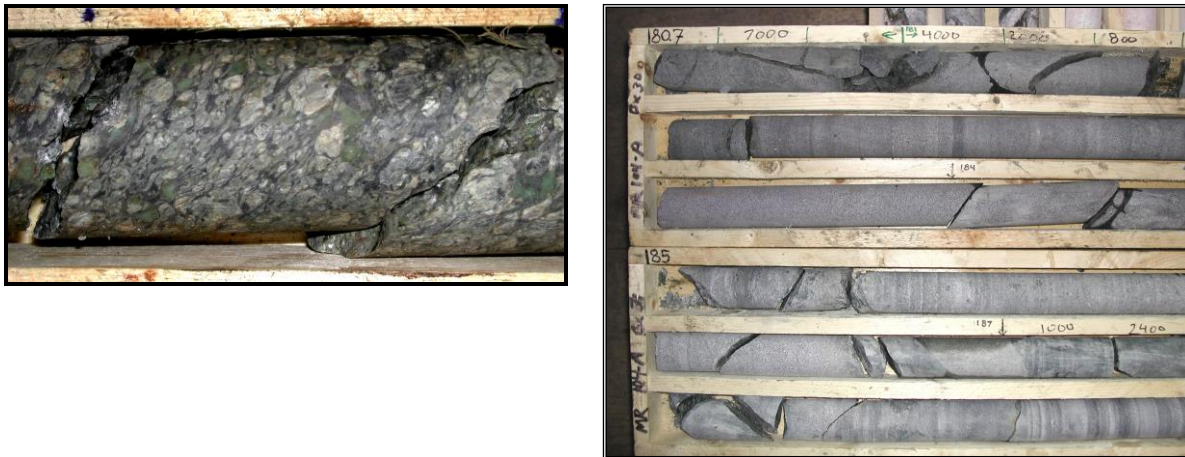
FIGURE 19: Representative textures and alteration in drill core: (a) Distinctive texture of the mylonitic microgranite. All drill cores in these pictures are NQ size (4.75cm diameter). (b) Grey-green Fe-illite chloritic alteration of the Fair Point Fm. Numbers written on the boxes denote counts per second using the SPP-2 (from Wheatley and Cutts, 2013).
